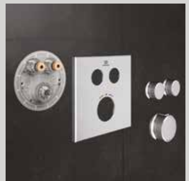
6. Slide the plate support over the cartridge and the diverter and screw into the right position. Then mount the visible design parts.
